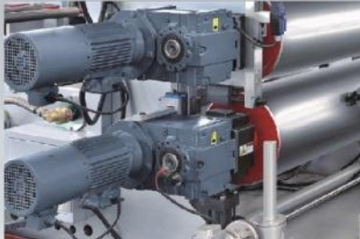
从下辊和中辊之间压料 Extrude Between By Down And Middle Roller
